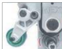
Guide roller prevents the pipe from detaching and eliminates vibration, so there's no need to place your hand on the pipe.
